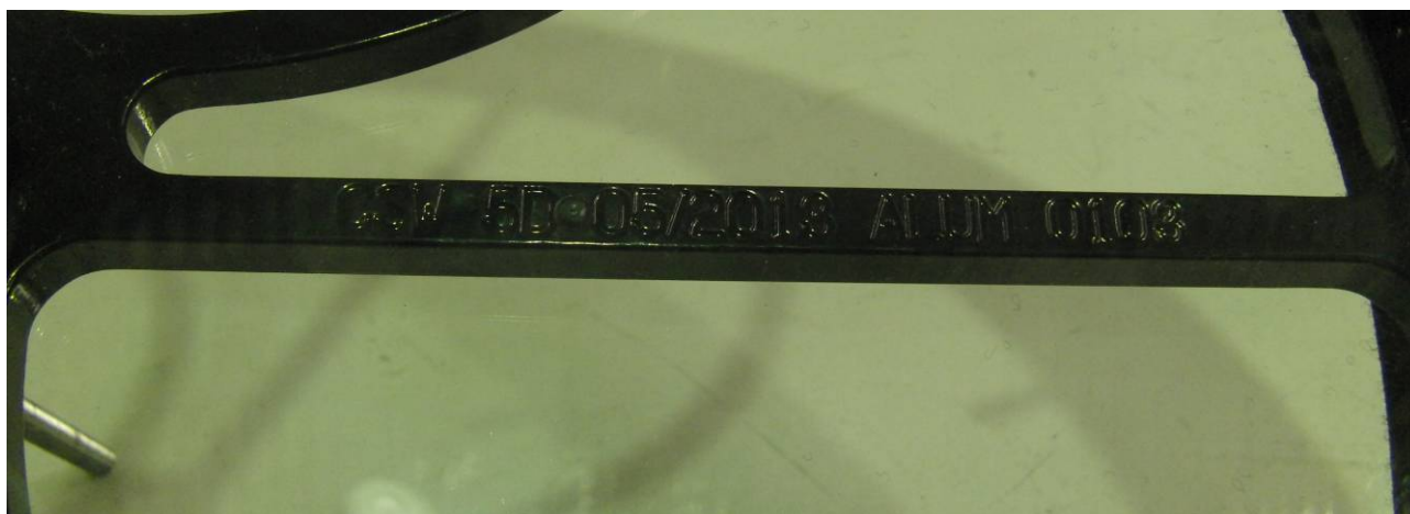
Figure 4 Markings shown on the tested wheels with the manufacturer (CSW), wheel model (5D) date of manufacture (5/13), material (Alum) and serial number (0103).
